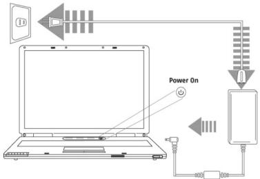
The power adapter is connected via a power cord to an AC outlet. The DC power lead from the power adapter is connected to the side of the Notebook.
